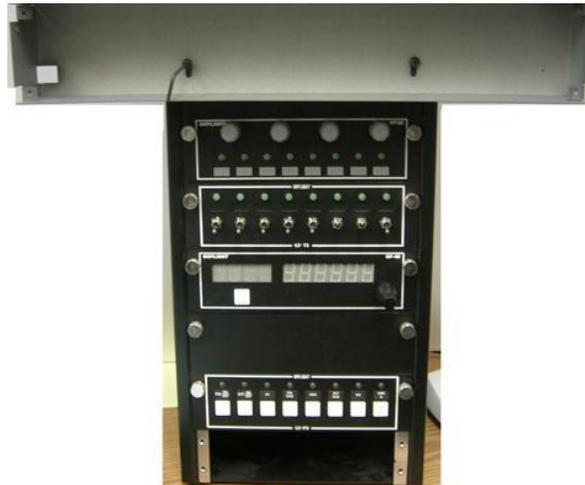
Place the electronic back into the case and attach with the four screws.
